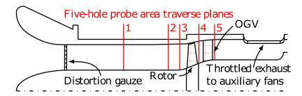
Figure 17. Meridional view of the BLI fan rig.
