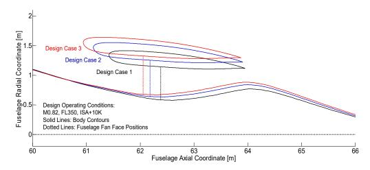
Figure 7. Changes in FF geometry of the Rev07 PFC design for different target FF shaft power.
