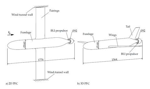
Figure 14. Schematics of the wind-tunnel models setup. Dimensions in mm.
