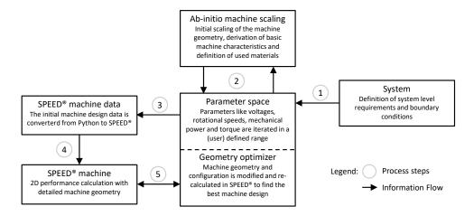
Figure 27. Basic electric machine design scheme.
