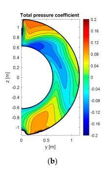
**Figure 10.** Contours of total pressure coefficient at the AIP. (a) PFC with axisymmetric aft fuselage, (b) PFC with aft-fuselage upsweep (Source: [58]).
