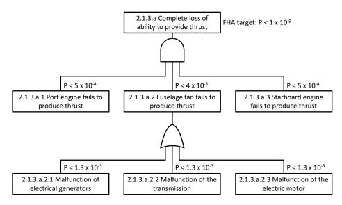
**Figure 30.** Example FTA for complete loss of ability to provide thrust for the CENTRELINE PFC aircraft.
