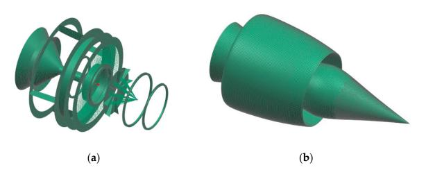
Figure 24. Finite element mesh for (a) internal structure and (b) skin of the aft-fuselage section.
