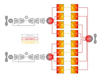
Figure 26. Overall propulsion system architecture (Source [81]).
