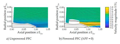
**Figure 15.** Time-averaged velocity field around the PFC aft-fuselage section of the 2D-PFC setup. Stereo-PIV measurements taken at  $V_0 = 20 \text{ m/s}$  and NPF = 0.
