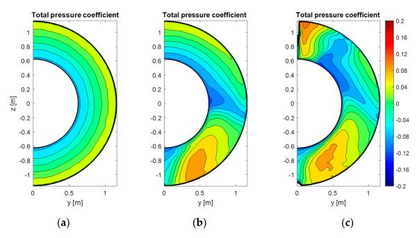
**Figure 9.** Contours of total pressure coefficient at the AIP. (a) bare PFC configuration, (b) bare PFC configuration + wing and (c) bare PFC configuration + wing + vertical tail (Source: [58]).
