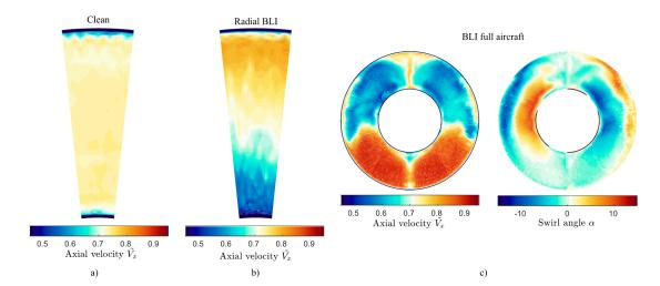
Figure 18. Measured inlet inflow behind the distortion gauzes: (a) Clean, (b) hub-low distortion, (c) full-aircraft configuration.
