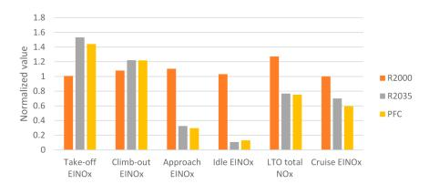
Figure 38. NO<sub>x</sub> emissions assessments results for the CENTRELINE R2000, R2035 & PFC aircraft.
