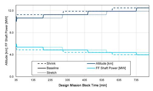
**Figure 36.** Cruise altitude and FF ideal shaft power profile for the PFC family members at Ma 0.82, ISA+10 K (adapted from [69]).
