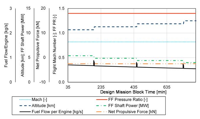
**Figure 35.** Simulated PFC aircraft specific performance characteristics recorded for the design mission cruise phase (adapted from [69]).
