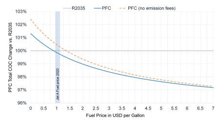
**Figure 40.** Fuel price study of CENTRELINE PFC versus R2035 design mission COC (adapted from [111]).
