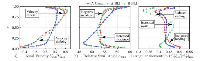
Figure 19. Measured spanwise distributions at the ADP of: (a) axial velocity, (b) relative swirl angle, (c) angular momentum.
