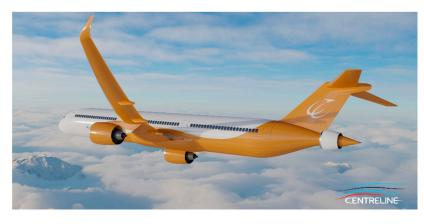
Figure 1. Artist view of the CENTRELINE turbo-electric propulsive fuselage aircraft design.
