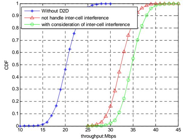
**Figure 4. The sum throughput of system only with cellular users, the system with cellular users and D2D users that not handle inter-cell interference, and the system with cellular users and D2D users using the proposed method.**
