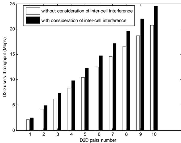
Figure 7. The D2D throughput with D2D number changed.
