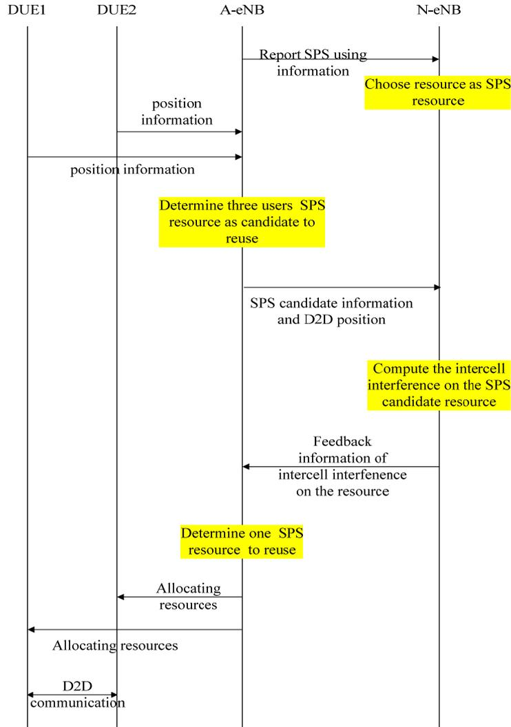
Figure 3. The proposed SPS resource reuse scheme.
