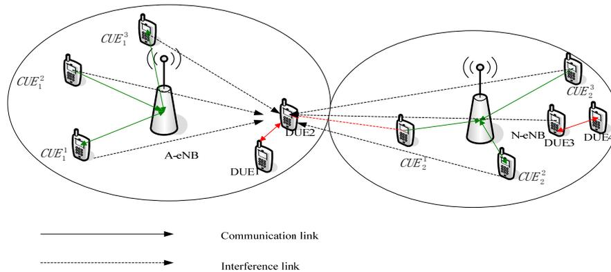
**Figure 1. An example of interferences in the LTE uplink.**
