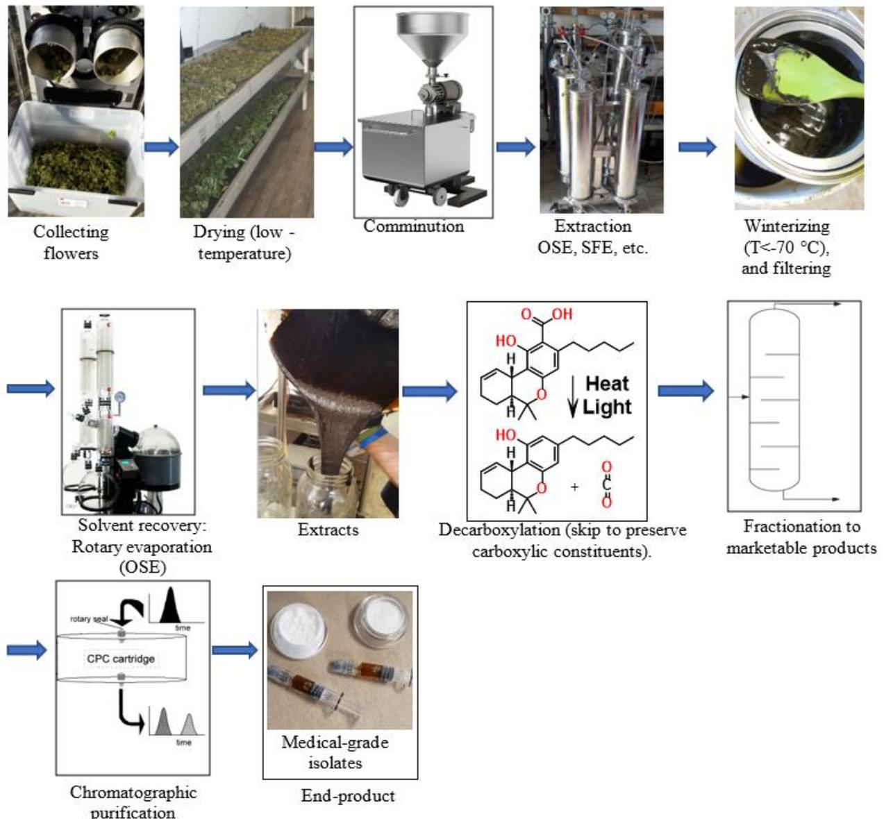
**Figure 2.** Process flow diagram showing the downstream processing steps needed to produce cannabinoids from *Cannabis sativa* L. OSE: organic solvent extraction; SFE: supercritical fluid extraction.
