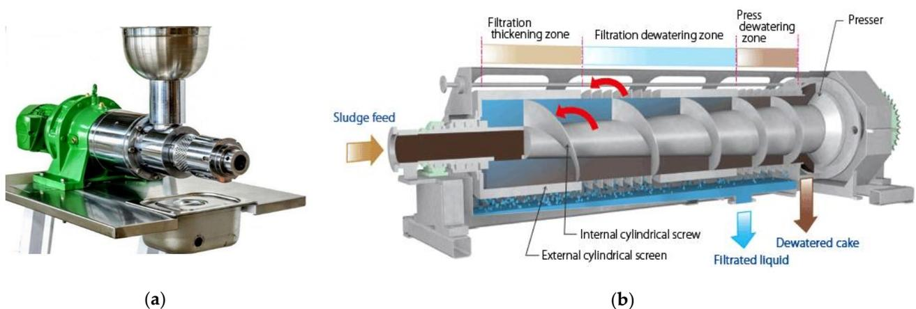
**Figure 5.** Two common types of screw expellers used for the cold pressing of hemp, (a) feed from top and (b) feed from front.
