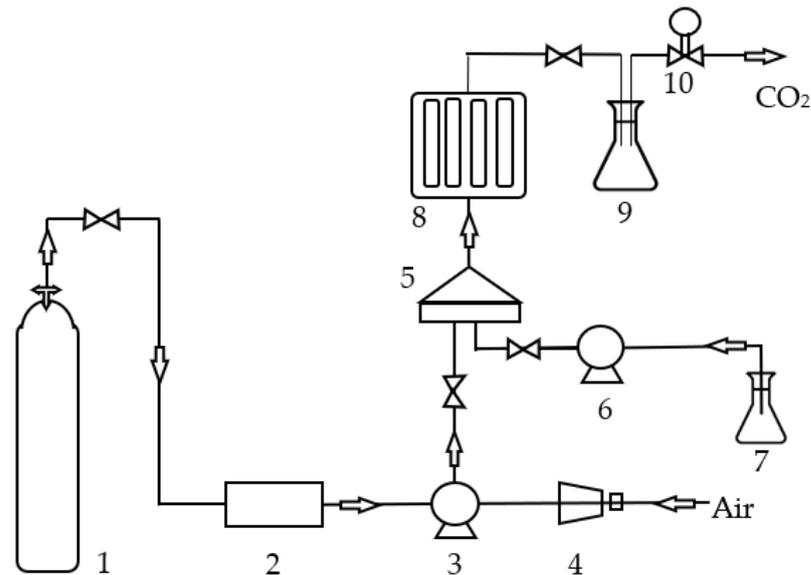
**Figure 3.** Schematic view of SC-CO<sub>2</sub> extraction unit. CO<sub>2</sub> cylinder (1); CO<sub>2</sub> cooler (2); booster (CO<sub>2</sub> pump-3 and compressor-4); mixer (5); co-solvent pump (6); co-solvent source (7); extraction unit (8); separation vessel (9); flow meter (10).
