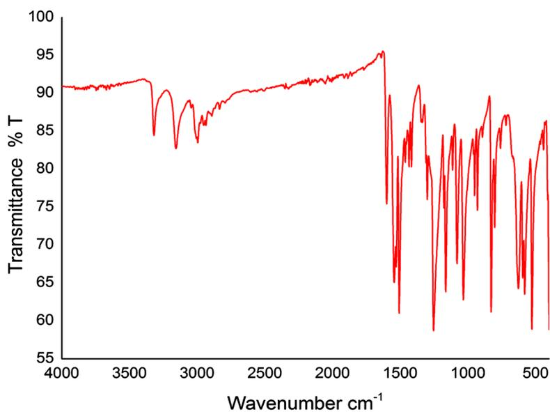
**Figure 3.** Infrared spectrum of PPEH.
