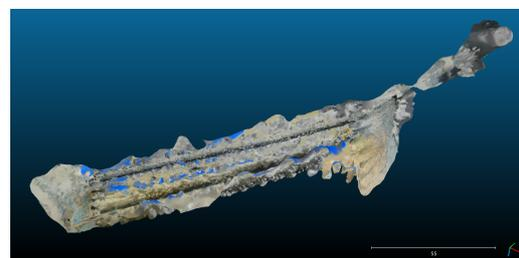
(a) The PIX4D resulting DSM that was built using images without embedded GNSS data.
